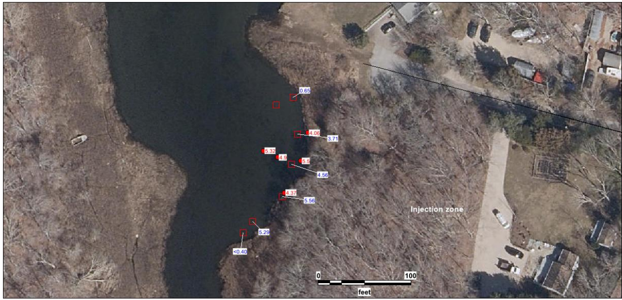
Figure 7: Porewater nitrate values in mg N/L from 2020 pre-PRB installation survey (red squares/blue text) and current values from fall 2023 monitoring (red circles/red text).
