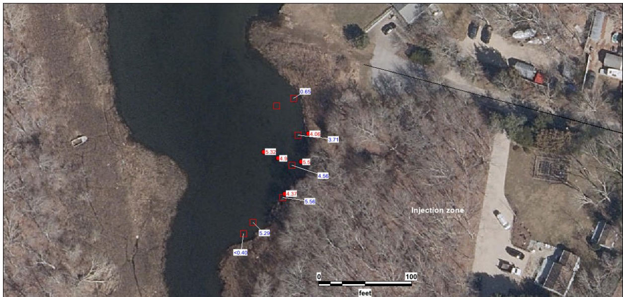
Figure 3 Porewater nitrate results for 2020 pre prb survey survey (red Square and blue text) and fall 2023 post PRB installation (red circles and red text) results in mg/l
