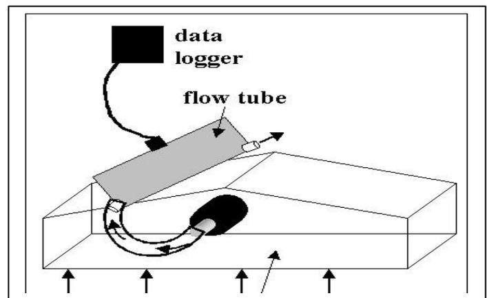
Figure 5- Ultrasonic Seepage meter system
