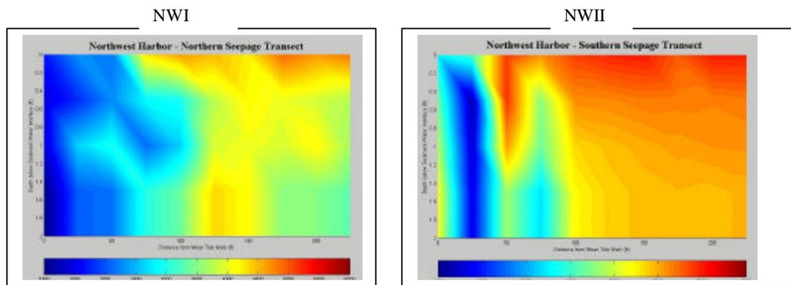
Figure 6—Resistivity Profiles. Note blue areas indicate areas of groundwater discharge
